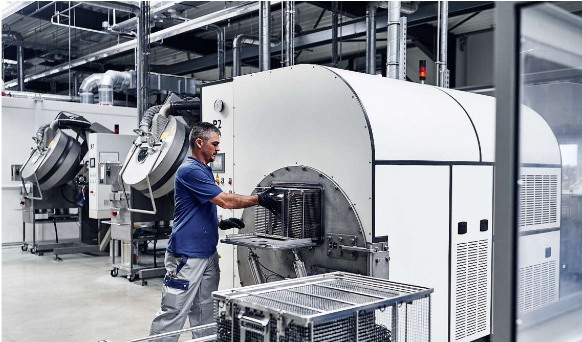
Image 6: Low-pressure plasma unit within APO's coating of small mass-produced parts
